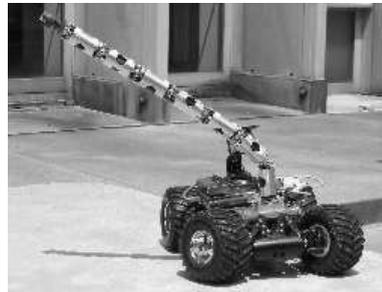
**Figure 1.7** The Carnegie Mellon snake robot Holt mounted on a mobile base.
