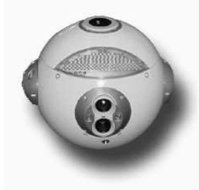
**Figure 1.1** NASA's Mini AERCam free-flying video inspection robot.
